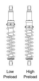
top of the shock and the threaded spring preload adjuster nut on the shock body. Failure to do so could cause the retainer to fall off when the suspension is fully extended.
